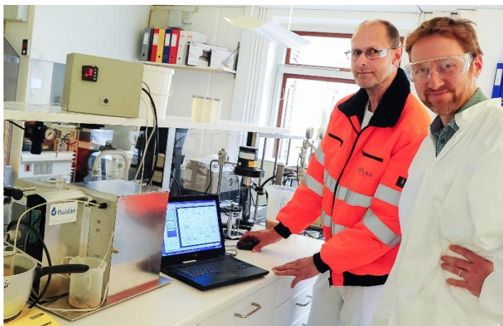
The inventor of RheoStream, Fridolin Okkels (right) is testing the flow cell at CP Kelco with Jack Hansen. The flow cell and the measuring system is in the metal box.
