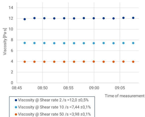
Continuous measurement of viscosity at three shear rates of wall paint. A new measurement at all three shear rates happens every other minute.
